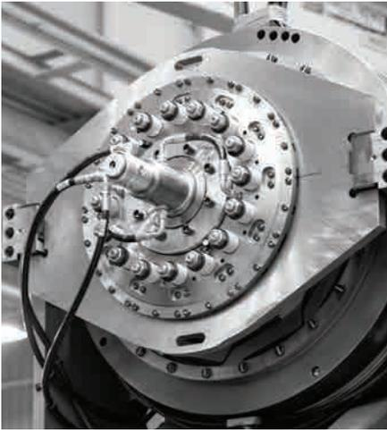
The Minster combination hydraulic clutch and brake provides the ability to single stroke at high rates while simultaneously providing unparalleled stopping time ability that is critical for high speed and in-die sensing applications.
