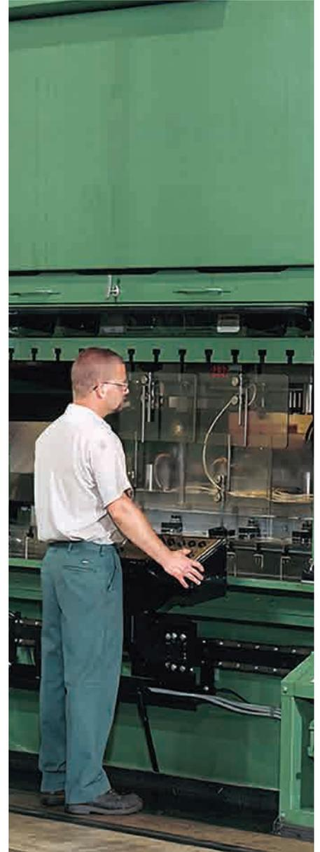
**3** Run progressive and transfer dies with high off-center loading.
